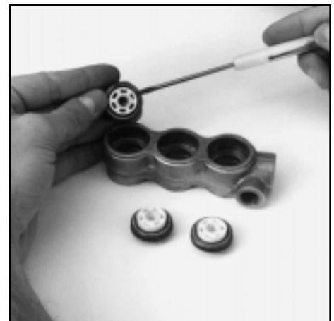
Installation of V-Packings
